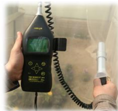
Microdust pro detector and how to measure airborne dust
